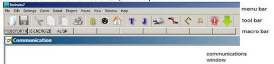
**Load/check settings:** On the menu bar click settings, open file. If you have an R12 or R17 click on R12R17.CFG; if an R19 click on R19.CFG. Axis names may be manually set using settings. **caps lock** – All ROBOFORTH commands are in upper case, ensure CAPS LOCK is on.
